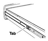
Press the tab DOWN on the RIGHT side and lift the tab UP on the LEFT side at the same time. Then pull drawer out another inch.
